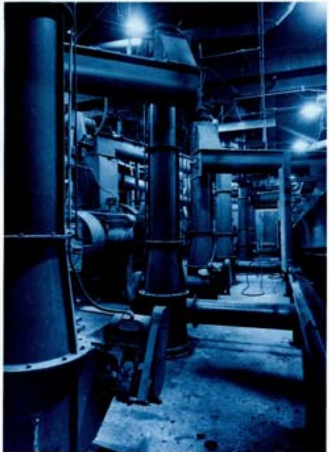
Rubber reclaiming operation uses high capacity, compact Screw-Lift and screw conveyor system to transport rubber back and forth between mills and screener.
