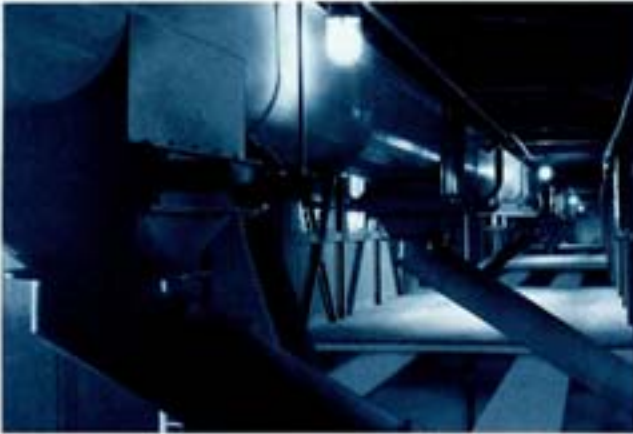
A Screw Conveyor installed in a large overhead operation. Space-saving features are apparent here. All parts of the system are enclosed yet readily accessible.
