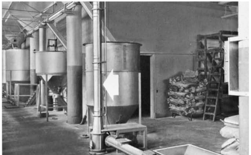
Screw-Lift and feeder moves material from floor to distributing conveyor over bins.
